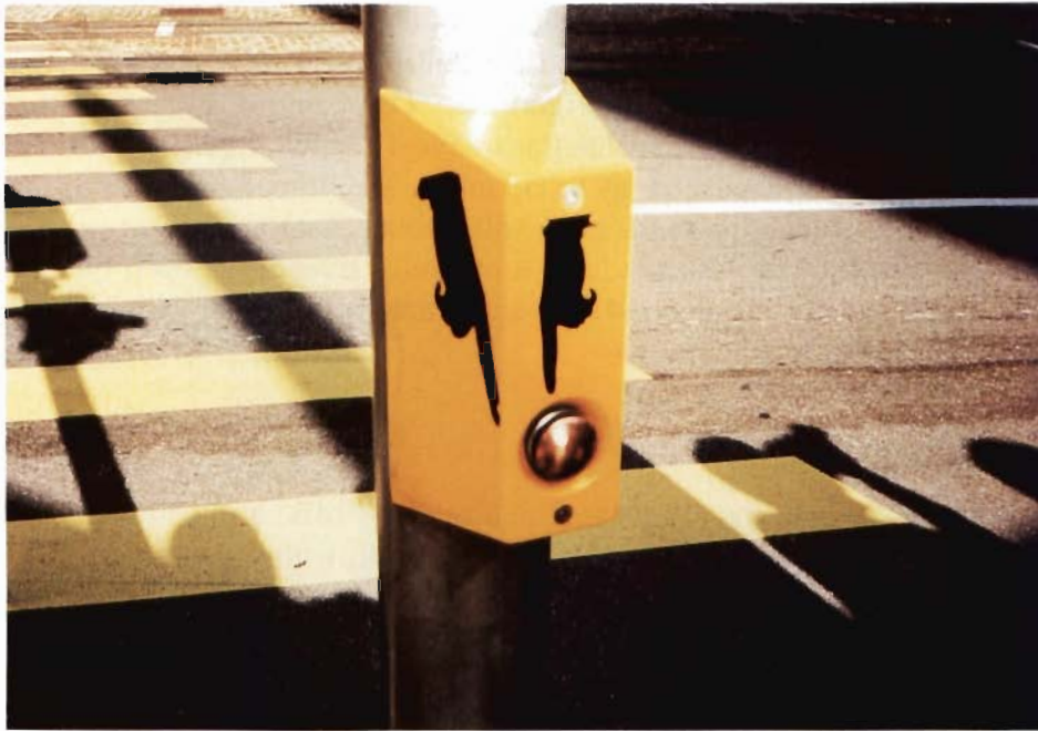
Figure 53. Pedestrian pushbuttons used at some Basel intersections.
