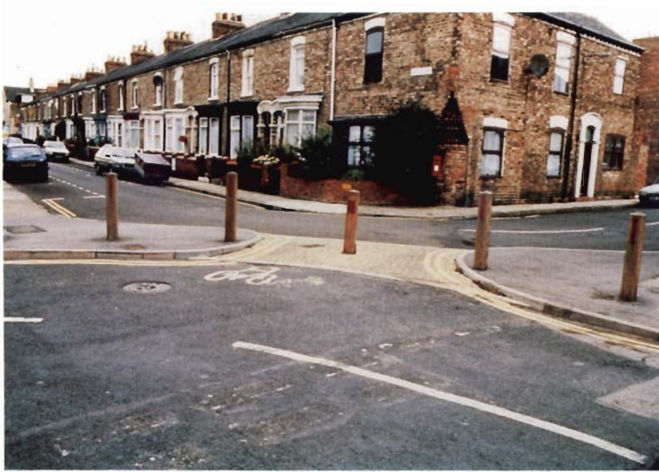
Figure 19. Diagonal motor vehicle diverter at a residential intersection in York, England.
