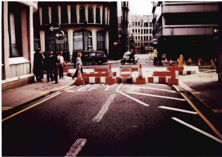
Figure 20. Temporary barriers used to block a street to motorized vehicles in London.
