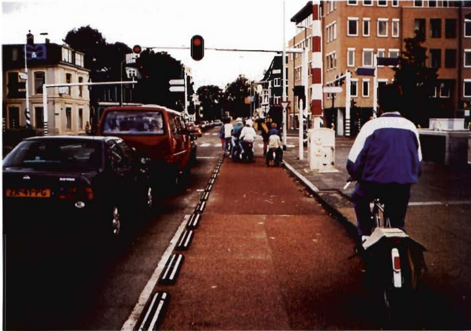
Figure 44. Rubberized C-curbs separate bicycle lanes from motor vehicle lanes in Frankfurt.
