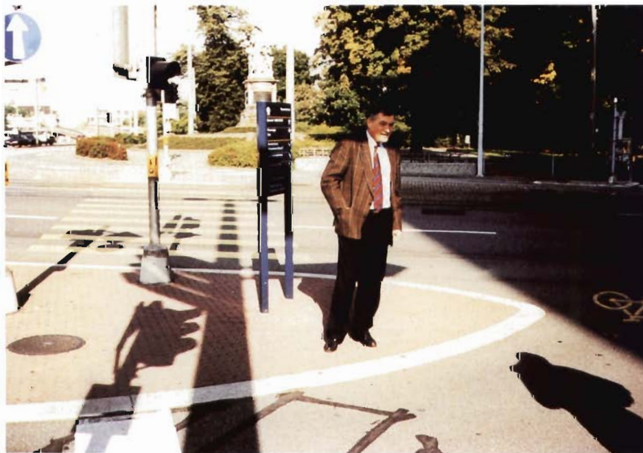
Figure 54. Pedestrian refuge island located in a wide street in Basel.
