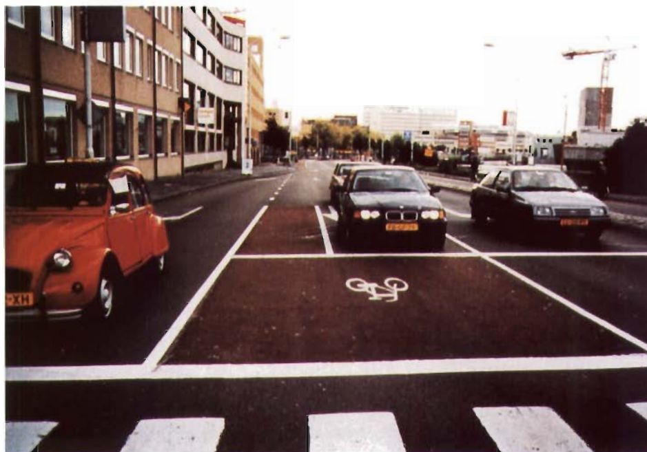
Figure 30. Advance bicyclist stop line at intersection in Groningen, The Netherlands.
