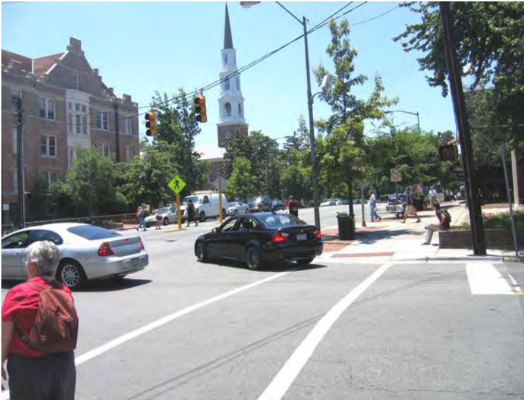
Figure 26. West side crosswalk on Franklin (crosswalk in the background with fluorescent yellow pedestrian warning sign) at Henderson St is set back from the intersection.
