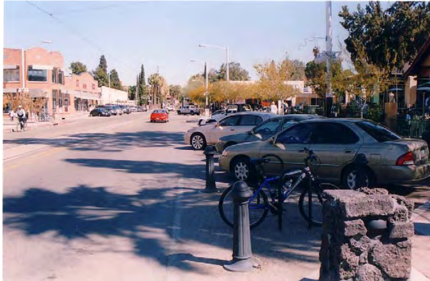
Figure 31. Reverse angle parking could increase amount of parking downtown and eliminate 'dooring' type crashes with bicyclists. Motorists are also positioned to better view oncoming traffic before pulling out of parking. (Photo from the PBIC Image Library)
