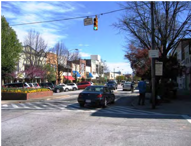
Figure 29. Downtown Hendersonville, NC streets have bulb-out sidewalk extensions. (Photo by Austin Brown)
