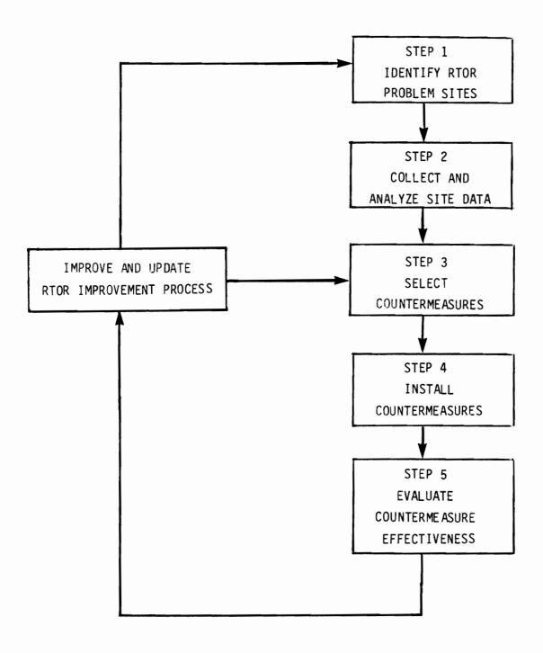
Figure 5. Flowchart of RTOR improvement process.
