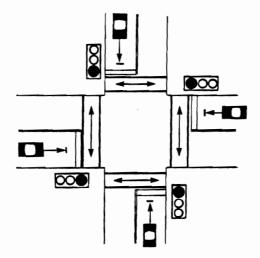
One type of exclusive pedestrian phasing is referred to as Scramble or Barnes Dance timing, where diagonal pedestrian crossings are also permitted. This crossing scheme is illustrated below with arrows illustrating the allowed pedestrian movements.
