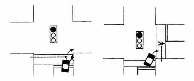
2. Interaction (I) - Neither the vehicle nor the pedestrian reacts, but the pedestrian is in a moving lane and is within 20 feet (6 m) of the RTOR vehicle (see sketches below).
