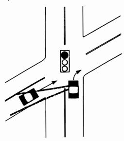
• Steep downgrade for oncoming cross-street traffic - If a RTOR vehicle turns in front of a "downhill" cross-street vehicle, it would be more difficult for a cross-street vehicle to stop (see sketch below).
