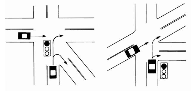
• A narrow lane to turn into and/or a turn radius of sharper than 90° - A difficult right turn maneuver may result for RTOR vehicles (see sketch below).
