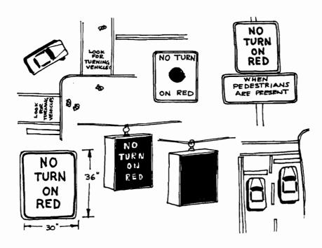
The most common countermeasure for RTOR-related problems that has been used to date has been to prohibit RTOR on an approach. Total as well as part-time prohibitions have been used. Countermeasures related to RTOR accidents may be used to accomplish several specific objectives, as follows:
