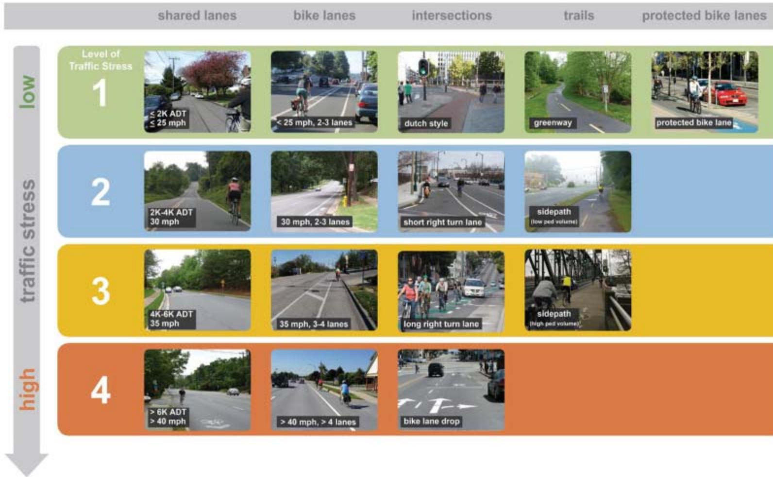
FIGURE 29: GRAPHICAL REPRESENTATION OF LTS SCORES BY BIKEWAY TYPE
